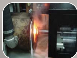
加熱淬火站及淬火液循環槽，設置線上回火裝製 Quenching and Tempering Station
