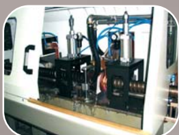
加熱淬火站及淬火液循環槽，設置線上回火裝製 Quenching and Tempering Station
