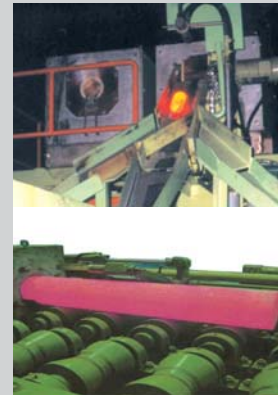
加熱爐體及工件輸送裝置 Induction Heater and Working Piece Driver System
